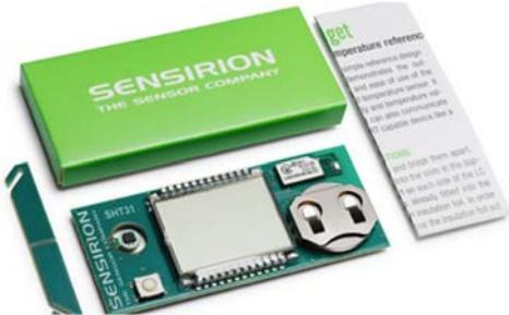
The SHT31 Smart Gadget is a reference design circuit board which demonstrates the outstanding performance and ease of use of Sensirion's humidity and temperature sensors. It not only shows humidity and temperature values on the display, but it can also communicate wirelessly with a Bluetooth Smart capable device like a smartphone. It comes with a battery.
